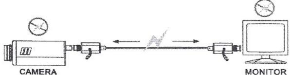
Recommend WT104PE Outdoor CAT5 UTP Twisted Pairs cable with PE jacket and steel wire, and use surge protector SP003-SP006 to avoid the damage of twisted pair system under lightning, thunderstorm weather environment.
